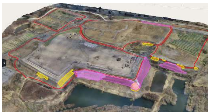
Aerial photograph of Crosby Warren landfill prior to the commencement of works showing project phase boundaries (red), slope movements (yellow) and existing remedial works (purple)
